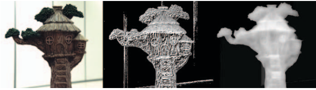
Fig. 3. Disparity refinement. (Left) Aligned color image. (Middle) EPI based Disparity Estimation. (Right) Our final disparity map.
